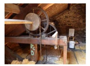
Fig.4: Lifting gear in the roof
